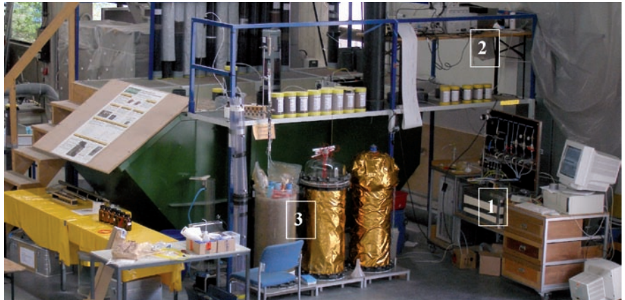
Figure 1: Small test container. Gas calibration system (1) and online reference analytics (2) used for soil gas measurements, and large water columns filled with contaminant-spiked water (3) for testing pumps and passive samplers. (Photo: VEGAS)
